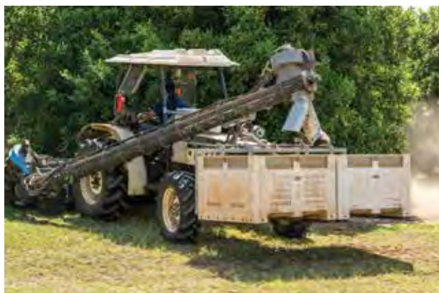
The smaller of Natara's harvesters where nuts are dehusked on board and emptied into Nally bins.
