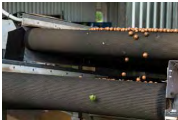
The double "waterfall" stick, rock and debris belt has significantly increased capacity.
