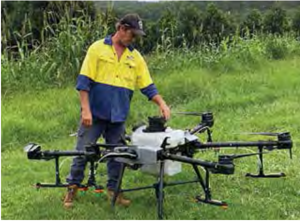
A drone with a 30 L payload was used by Scott Fisher from Skytech Solutions to apply chemistry.
