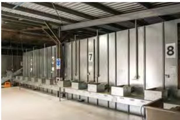
New 10 t storage silos where nuts are dried down to about 10% moisture before being consigned to the processor.
