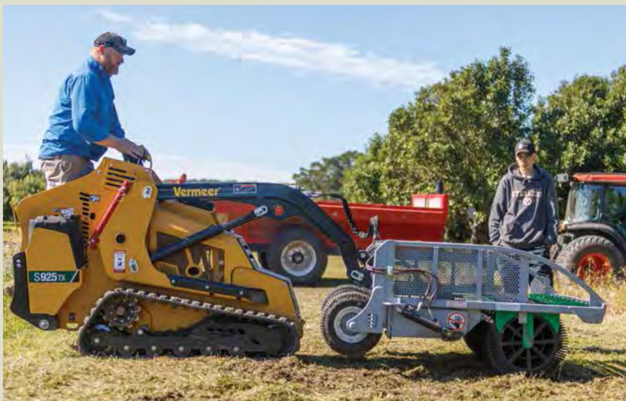
The mini skid loader has been fitted with a hybrid harvester, which has a holding bin with a 140 kg capacity. In the photo are Graham Wessling (left) and Zac Sullivan, a staff member.
