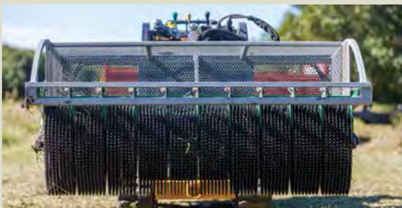
Ten off-the-shelf finger wheel packs have been fitted to the harvester and can be easily cleaned.
