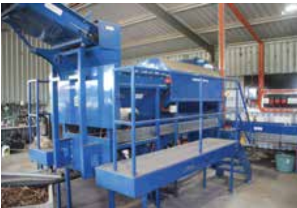
A four-head dehusker with stick and air sorter has resulted in significant improvement in productivity so that Ian can now process 10 t of NIS a day.
