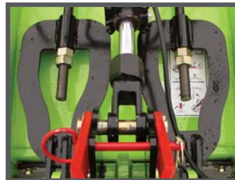
Dual levelling rods with floating hitch
